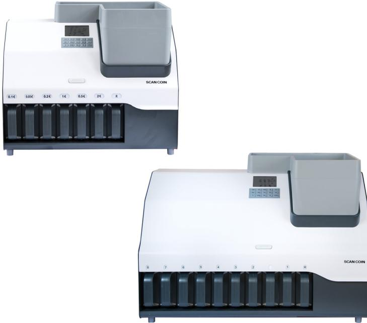
**DTC-9** – the largest in the group has nine sorting positions and one reject position. All positions has exchangeable labels. DTC-9 can sort maximum 9 denominations. DTC-9 Active is equipped with an extra solenoid to count and separate a denomination too close in diameter or to separate a currency.
